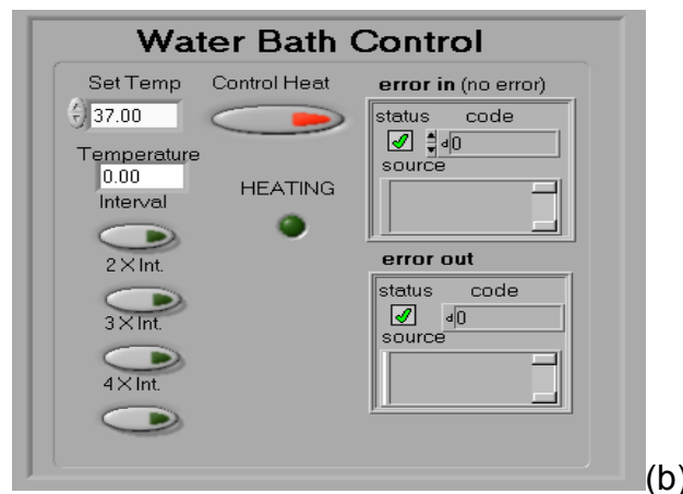
Figure 3.3-6: The water bath control VI block diagram (a) and front panel display (b).
